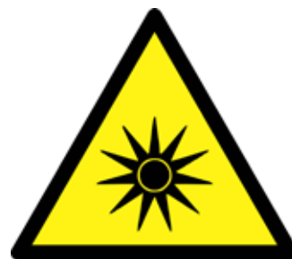
Figure 1. Optical radiation hazard warning sign [ISO 7010-W027 (2011-05)]. The warning sign should be placed on the lamp product with the explanatory marking.
